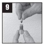
Place Extermination Cartridge into Firing Barrel cavity as shown. Reinsert Firing Barrel into MOLECAT.®
